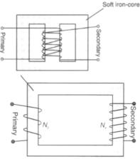
Principle: Step-down transformer is made up of two or more coil wound on the iron core of the transformer. It works on the principle of magnetic induction between the coils. When the current flowing through the primary coil changes, an emf is induced in the secondary coil due to the change in magnetic flux linked with it.
