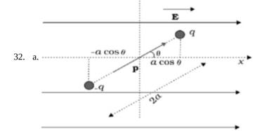
Since torque acting on dipole
